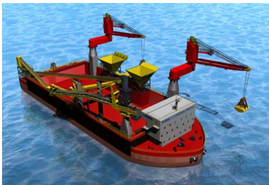
Figur 5-9: Floating terminal – Bulk Prosperity (20.000-30.000 t/dag)
