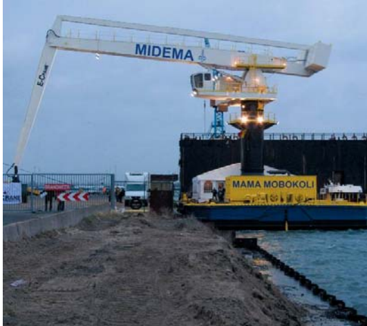
Figur 5-10: Floating terminal, Mama Mobokoli (400 t/h)
